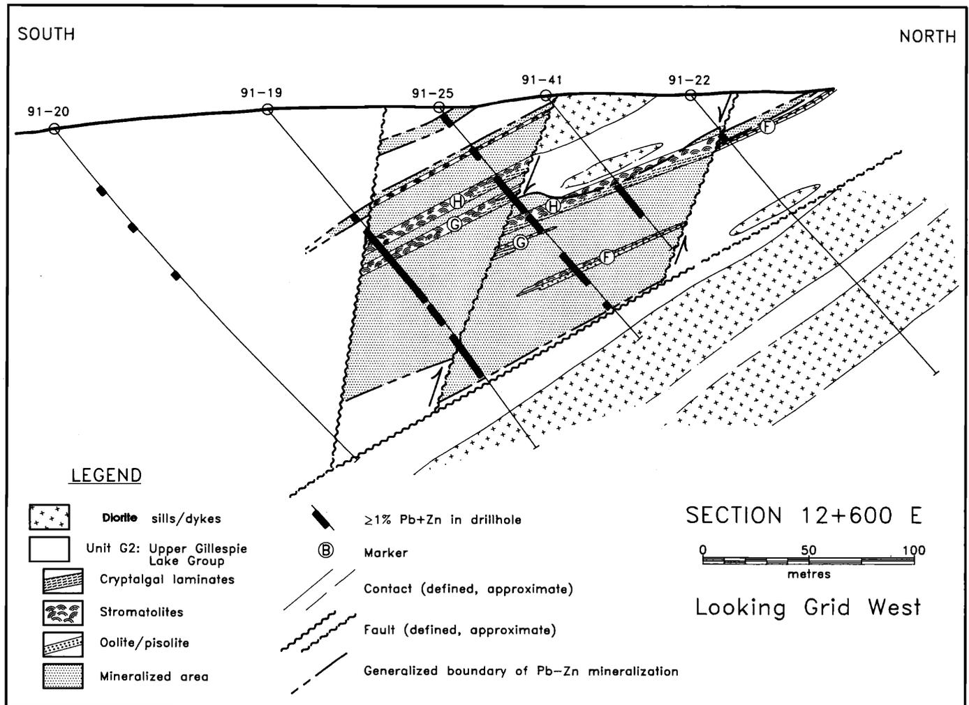
FIG. 4. Geologic cross section of the east zone (section 12 + 600 E, Fig. 2) showing marker beds F to H, Blende property, Yukon Territory. F = coarsening-upward oolite overlain by stromatolites. G = sphalerite-rich stromatolitic dolostone. H = pyrite-rich stromatolitic dolostone.
