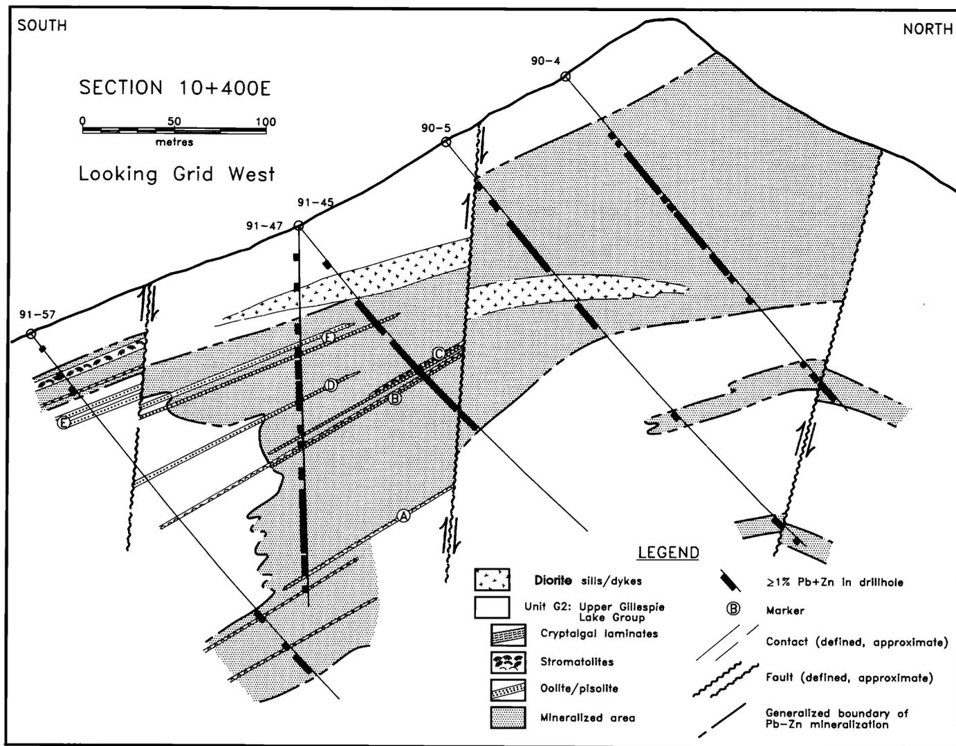
FIG. 3. Geologic cross section of the west zone (section 10 + 400 E, Fig. 2) showing marker beds A to E, Blende property, Yukon Territory. A = sphalerite-rich stromatolitic dolostone. B = coarsening-upward oolite overlain by stromatolites. C = coarsening-upward oolite overlain by club-shaped stromatolites. D = medium gray dolarenite with silicified oolite patches. E = interbedded oolitic dolarenite and dolosiltite.
